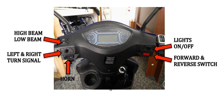
VII. Use the thumb throttle to GO as well as control the speed. The speed and the battery indicator are located on the dash. We advise driving at low speeds until you are comfortable using the scooter. Keep in mind as soon as you release the throttle the machine will automatically brake and come to a stop.
