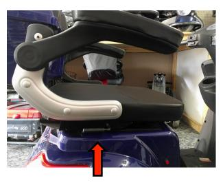
III. Before turning on the machine check whether the scooter is in the Drive (D) function or the Reverse (R) Function, adjust accordingly using the red switch shown below. Always to come to a full stop before switching between Drive and Reverse.
