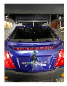
IX. In order to open the rear-box storage insert the key into the lock mechanism, hold the key in the open position and lift up the top of the storage box.
