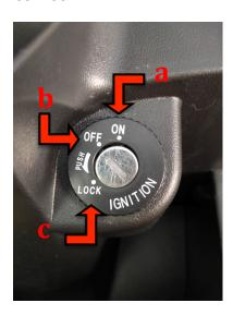
IV. To engage the front wheel lock you must turn the handlebars all the way to the left, push the key in then turn your key to the **c** position. To dis-engage ensure the handlebars are turned all the way to the left and turn your key to the **a** or **b** positions.
