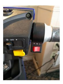
VII. Use the throttle to GO as well as control the speed. When the throttle is turned towards the rider the ebike will go forward. The speed and the battery indicator are located on the dash. We advise diving at low speeds until you are comfortable riding to the ebike.
