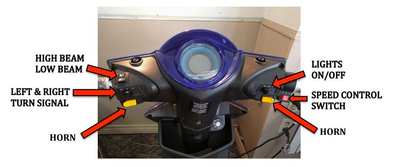
VI. The speed control switch controls and limits the speed of your ebike. There are three speeds; H is high speed, M is medium speed and L is low speed. L is ideal for initial pickup, once you have reached top speed switch to M then H.
